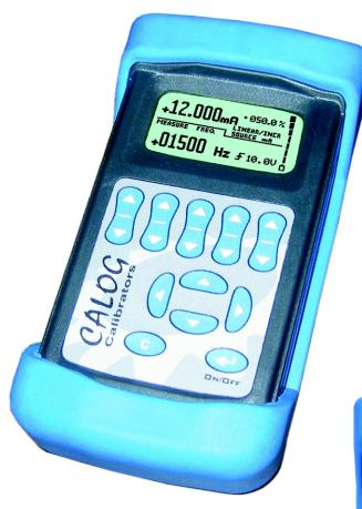
The CALOG- PRO is a high precision, multi-function, hand-held calibrator designed for the process control industry. The unit is capable of displaying measured values, sourced values or split screen measure and source simultaneously. Variables are milliamps, volts, millivolts, frequency and counts. It is especially suitable for PLC and SCADA applications. Circuit continuity can be measured with both audible and visual indication.
