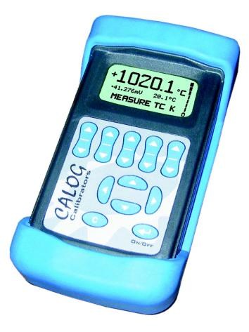
The CALOG - TC is a high precision, multi-functional, hand-held calibrator suitable for the process control industry. It's speciality is thermocouple based instruments. It measures and sources, thermocouple, millivolts and milliamps. It can measure DC Volts and continuity. The trend feature is ideal for graphing temperature profiles and PID controller optimization. It's small size, long battery life and high precision make the CALOG - TC ideal for industrial field or workshop calibration.
