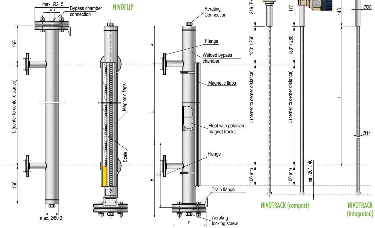
The end of the probe should extend the inverse polarized error indication flaps with 20 / 40 mm (0.78 / 1.57"). The supplied aluminum spacers are fixed with hex socket set screws and they are mounted to the bypass tube with pipe clamps. In case of the high-temperature type there is a ceramic fiber insulation blanket between the magnetostriuctive probe and the bypass tube.
