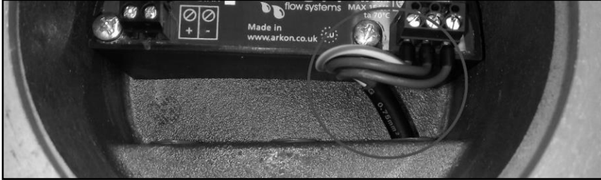
Pic. 1 round cross cut cable properly connected inside of MAGX2 IP68 housing
