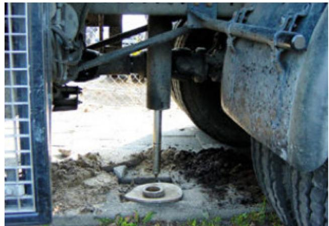
*The cone is pressed into the ground*
