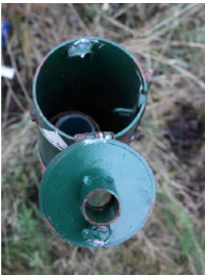
*Integrated GSM-2\* remote transmitter*
