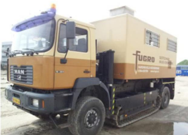
*Special trucks used for cone penetration testing*
