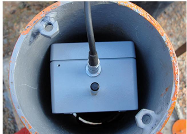
GSM-2 box\* remote transmitter with data logger
