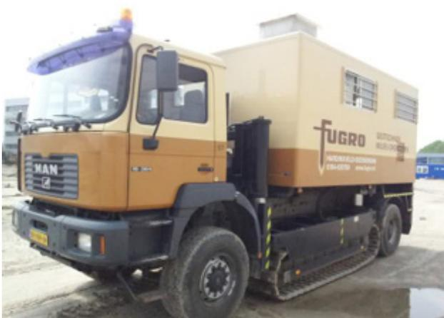
Special trucks used for cone penetration testing
