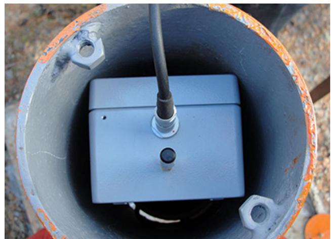
GSM-2 box\* remote transmitter with data logger
