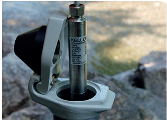
*Sensor in a DCX-22 AA data logger*
